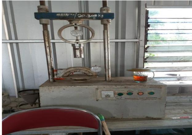
Gambar 7. Alat Uji *Marshall* (Sumber :Merza okta vianda,2020)
