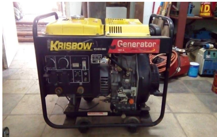
(Gambar 7. Mesin generator)
