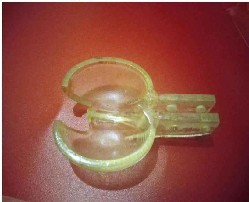
Gambar3.2 Bucket TurbinPelton
