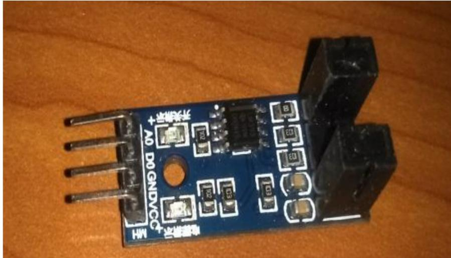
Gambar 3.4 Photo Sensor Interuptor
