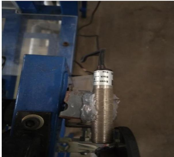
Gambar 3.5 Photo Sensor Interuptor
