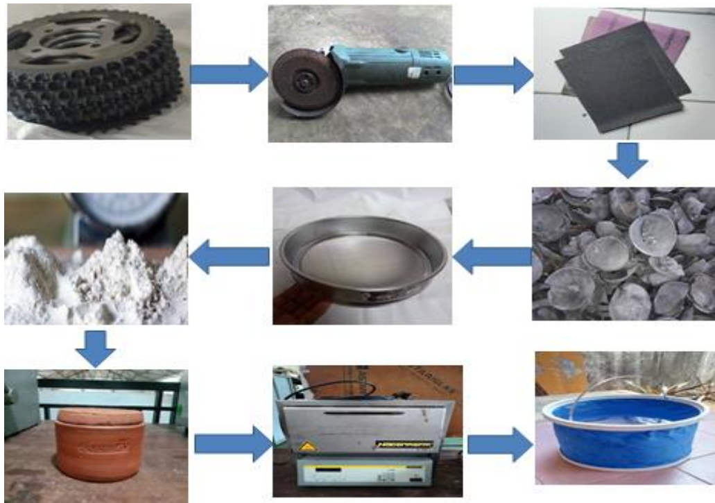
Gambar 24 Proses carburizing (Sumber :Dokumen pribadi)
