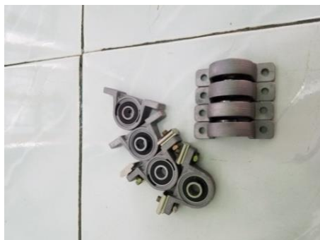
Gambar 40. Bearing shaft support (Sumber: Dokumentasi Pribadi)
